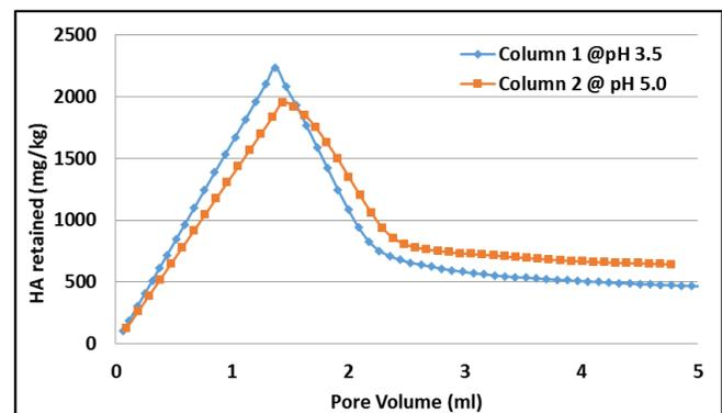
**Fig 4. Retention of humic acid in the columns at different pH values**
