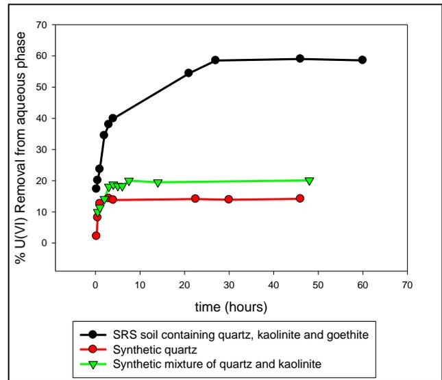
**Fig 2. U (VI) removal by different mineral phases present in SRS sediments as a function of time. Results indicate that goethite plays the major role in U (VI) sequestration.**
